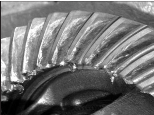
Burned ring & pinion
